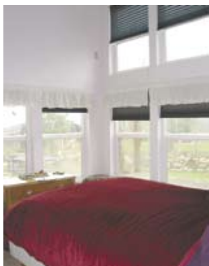
Above: Large south-facing windows admit an abundance of sunlight, eliminating the need for artificial lighting during the day, and providing heat during the winter. In the summertime, drawing the shades prevents the rooms from overheating.
