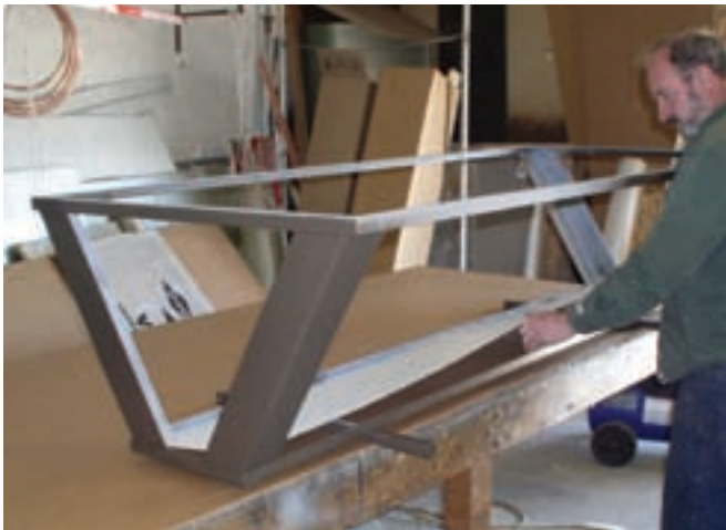
The welded steel frame of a tank-type batch water heater.
