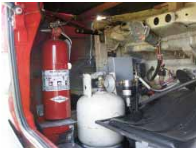
An LPG tank adds power and efficiency by mixing propane with the intake air prior to combustion.
