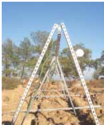
Sighting down the arrays, the pivot arms should look continuous.
