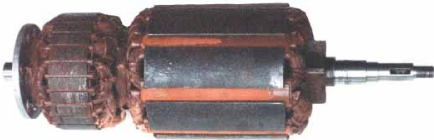
The rotor of a brushless alternator: The smaller section at left is the exciter armature; the larger section at right is the main alternator field. The diodes are mounted on the aluminum disk at the left end.
