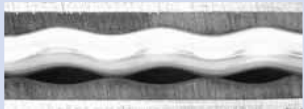
Cut-away view of the helical rotor mechanism, showing cavities that form between the rotor and the rubber stator.
