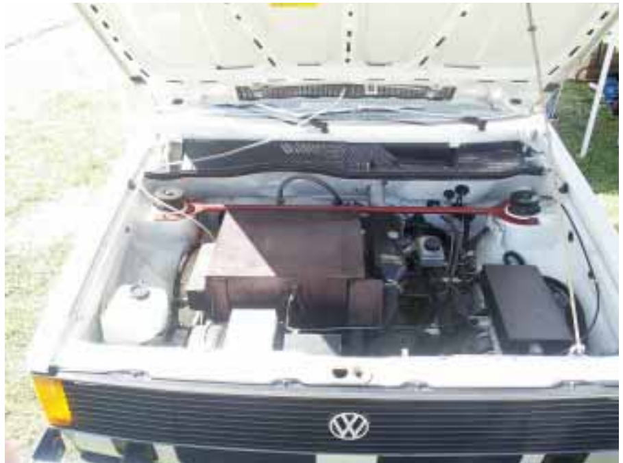
Under the Rabbit's hood—an electric power plant perfect for around town use, with up to 40 miles total distance between charges.
