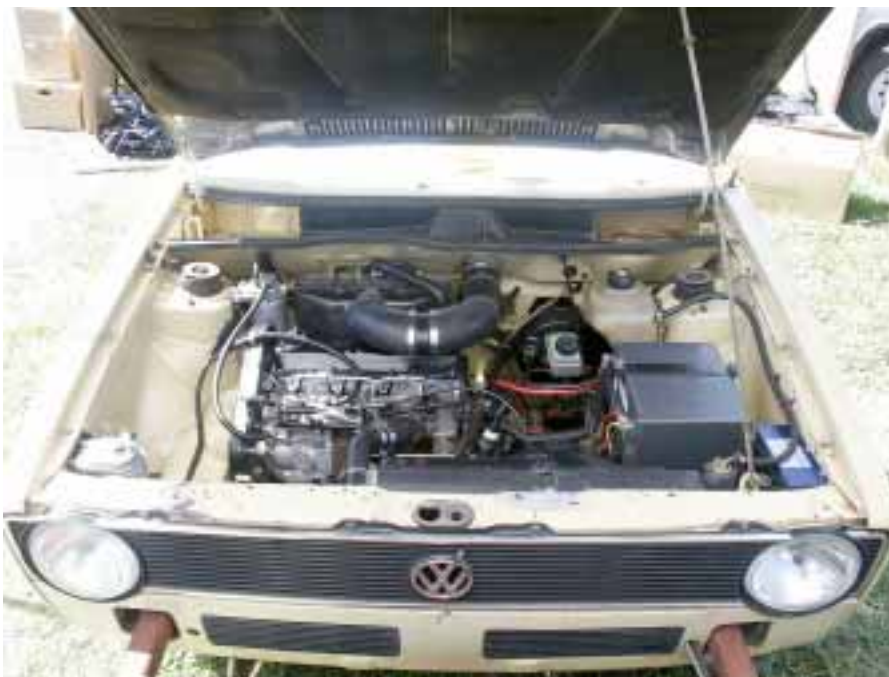
Inside the trailer—a diesel power plant including fuel tank, automatic transmission, and "front" wheel drive adds significant range to the EV.
