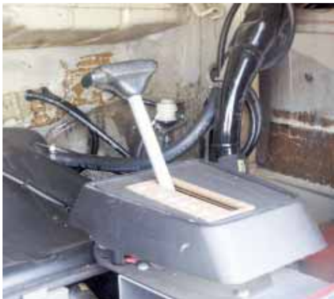
A stock Rabbit automatic transmission makes operation simple. Gear ranges and Park/Neutral are selected by use of a familiar shift lever mounted in the trunk of the trailer.
