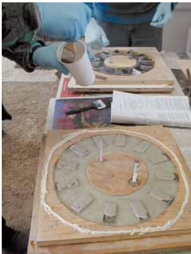
Close-up of students casting magnets in resin during SEI’s Homebuilt Wind Generators workshop.
