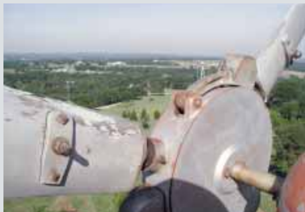
The hub of an old Jake showing the unique flyball governor that controls blade pitch.
