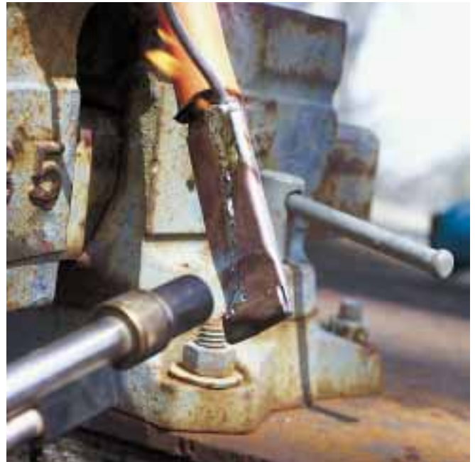
Steps 9 & 10: Gently secure the cable in a vise and flow solder into the tubing until full. Let cool before handling!
