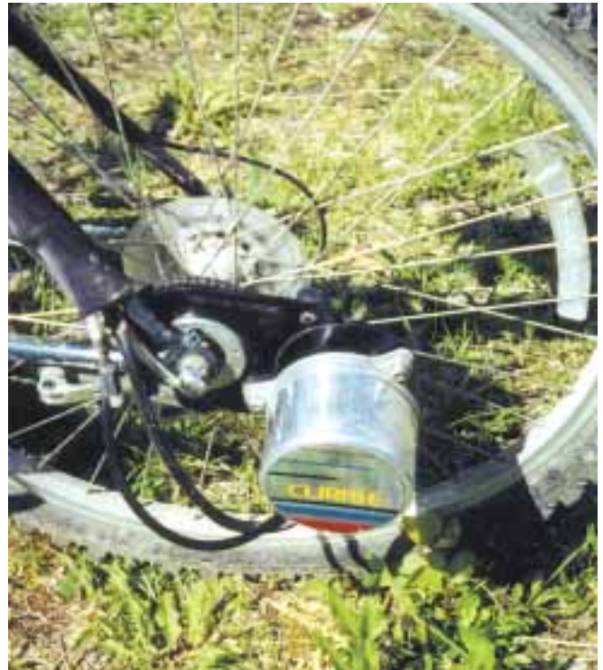
The motor and drive train mount to the bike's rear hub.
