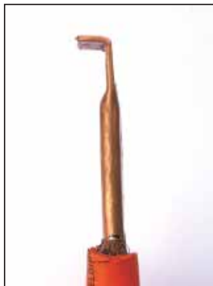
Step 8: Fold the end over in a vise, shown half completed.
