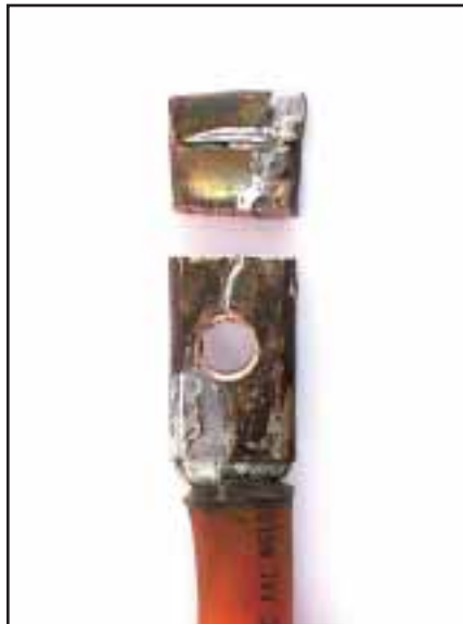
Step 13: Trim off the excess part of tubing that contains no cable.
