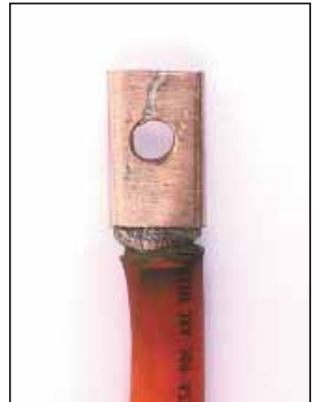
Step 14: Polish and brighten the connector for good contact.
