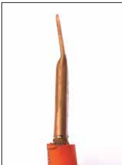
Step 7: The end of the tubing without cable gets pounded flat.
