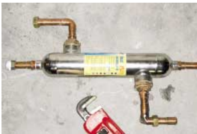
The liberal use of threaded unions allows for easy removal of components for repair or replacement.
