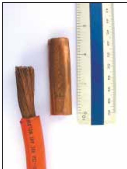
Steps 1-3: Strip insulation from cable and cut copper tubing to length.
