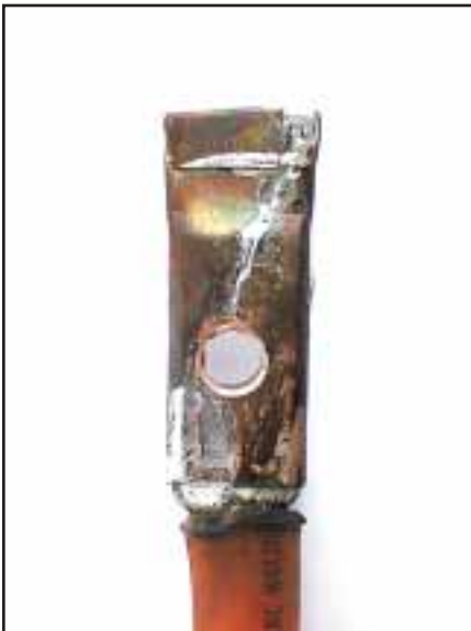
Step 12: Locate and drill the bolt hole.
