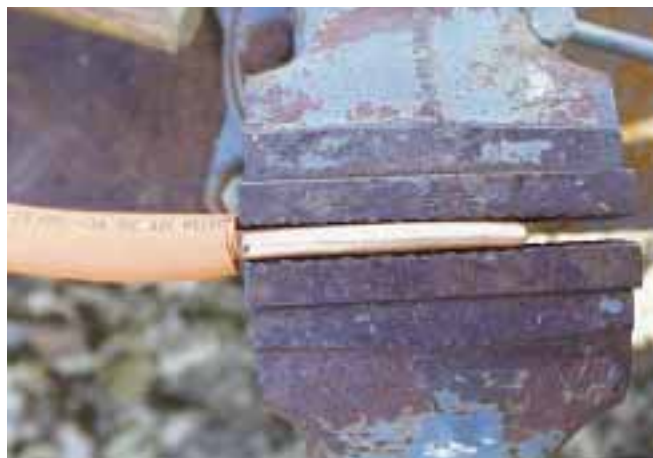
Step 6: Flattening the tubing in a vise.
