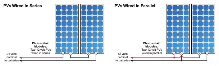
blocks. Here the positive output wires are paralleled or connected together. The negative output wires are also wired in parallel using a combiner block that's electrically isolated from the positive parallel block. See the right-hand diagram on page 36.
