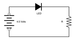
Starting at the lower left with zero, going clockwise, we add 4.5 for the battery, subtract the voltage used by the LED, then, by subtracting the voltage used by the resistor, we'll be back to where we started, with zero:
