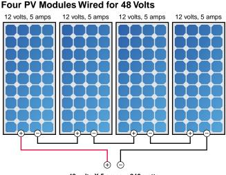
48 volts X 5 amps = 240 watts
