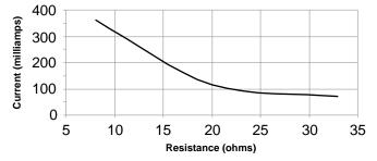
In this case, three resistor values were used against three LEDs and the voltages measured across the resistor, and the conclusion is that once the current exceeds 30 milliamps per LED, a large proportion of the electrical energy would
