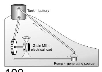
In the diagram below, the pump is analogous to the generating source—PV, wind generator, etc. The tank is analogous to the battery in a simple DC system. The plumbing represents the wires, and the water represents the charges or electrons that flow in the wires.
