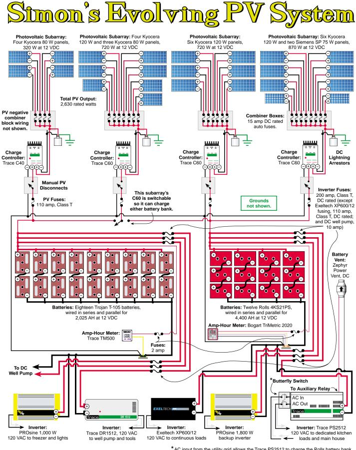
\*AC input from the utility grid allows the Trace PS2512 to charge the Rolls battery bank. The butterfly switch assures that the grid is only used for battery charging. This system isn't utility-intertied.
