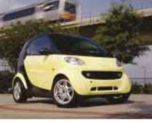
It also will be fully U.S. safety certified, crash tested, and highway capable. The chassis incorporates a sturdy cage for passenger safety. Top speed will be about 70 mph (113 kph), with a range of 60 to 70 miles (97–113 km).
