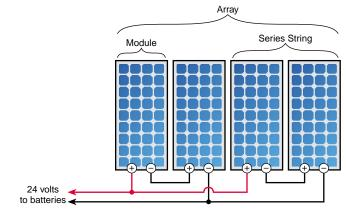
current decreases, and vice versa. The fact that you can make series and parallel connections allows you to specify the voltage and current of your PV system. It gives you some control over the power formula.
