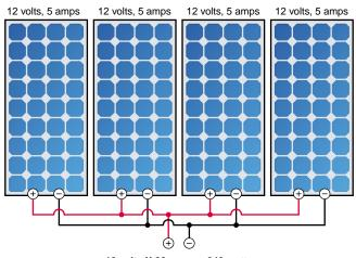
12 volts X 20 amps = 240 watts
