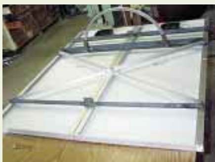
The pivoting assembly with two PV panels bolted to angle iron crosspieces and aluminum cross bracing. Note the pivot points on the outer angle irons, and the half-bicycle rim mounted to the center angle iron.
