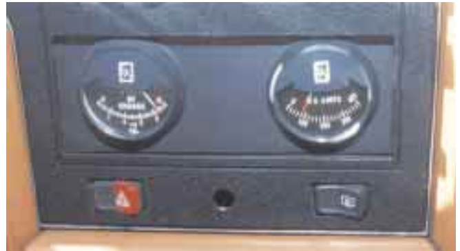
Watch your gauges—as volts go up, amps go down.
