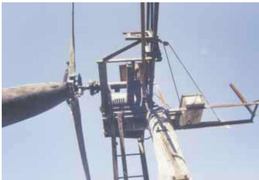
Looking up from below: the genny's tail structure is folded to the side.
