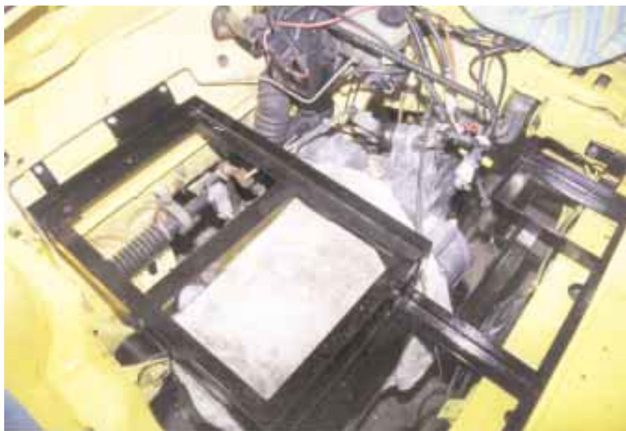
A split-level bridge rack supported on the right by the original bumper bracket bolts, and in the rear by the mount plate on the firewall.
