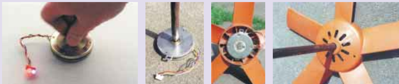
From left to right: Testing the stepper motor with LEDs. Fitting the windmill's shaft onto the motor. Installing the stepper motor inside the fan. Shaft attached to the fan, and facing the right direction.
