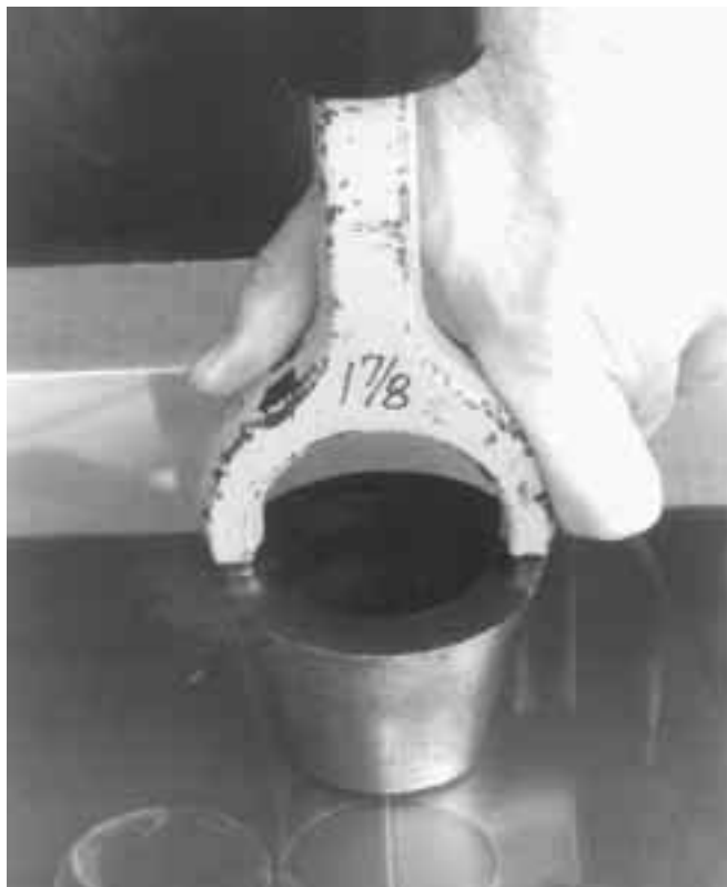
Above: Punching PEM from sheet with arch punch.
