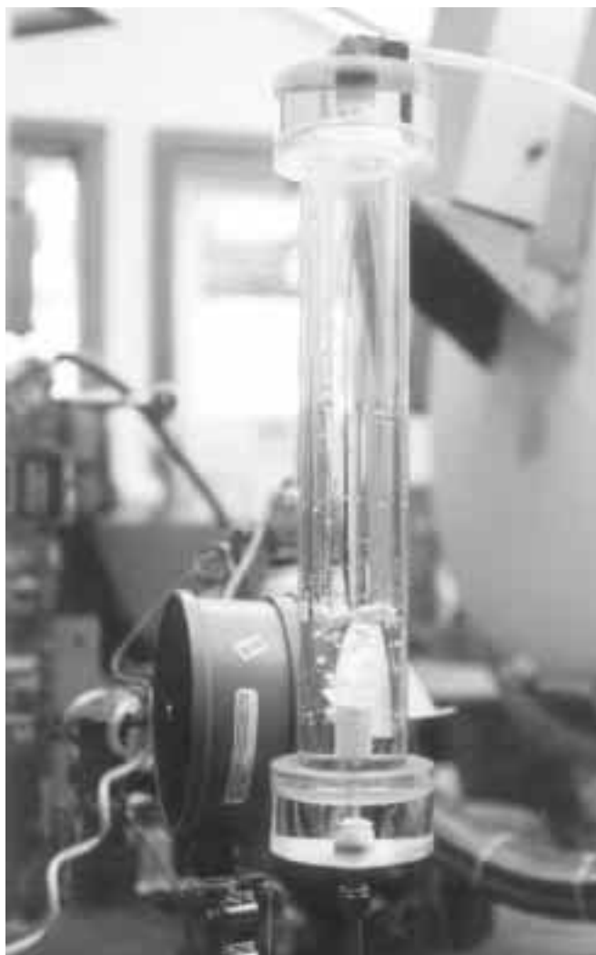
Above: H 2 humidification bubbler. Photo by Walt Pyle
